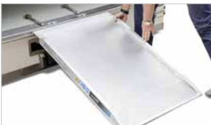
[10] Locate ramp on rear door step rail.
